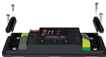
B Removing the strain reliefs
