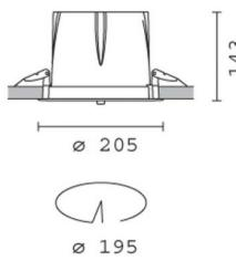
**Product code**MN96: recessed luminaire Ø 205 - neutral white passive dissipation LED - integrated DALI control gear - flood **Attention! Code no longer in production****Technical description**
