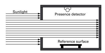
Optimal light conditions for actual value correction. Measurement results at the installation location or at the reference area are affected equally by natural light.
