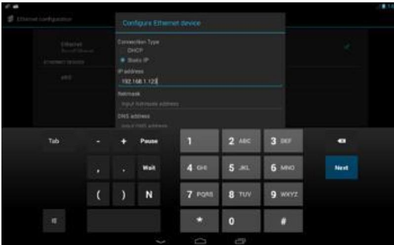
DHCP means Dynamic Host Configuration Protocol and the possibility to use, when available, the configuration service of the network card with dynamic IP. In this way our computer can be used to access the network.
