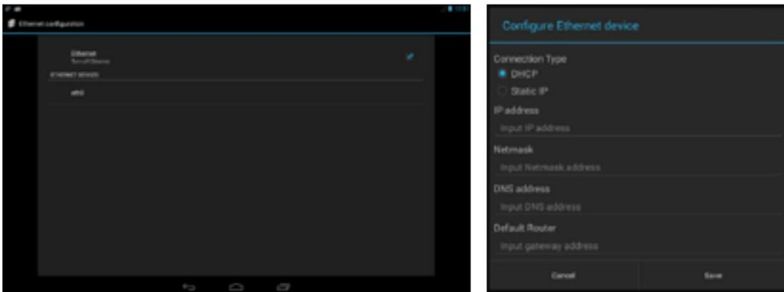
DHCP means Dynamic Host Configuration Protocol and indicates the possibility to use, when available, the configuration service of the network card with dynamic IP. In this way our computer can be immediately used for access to the network.
